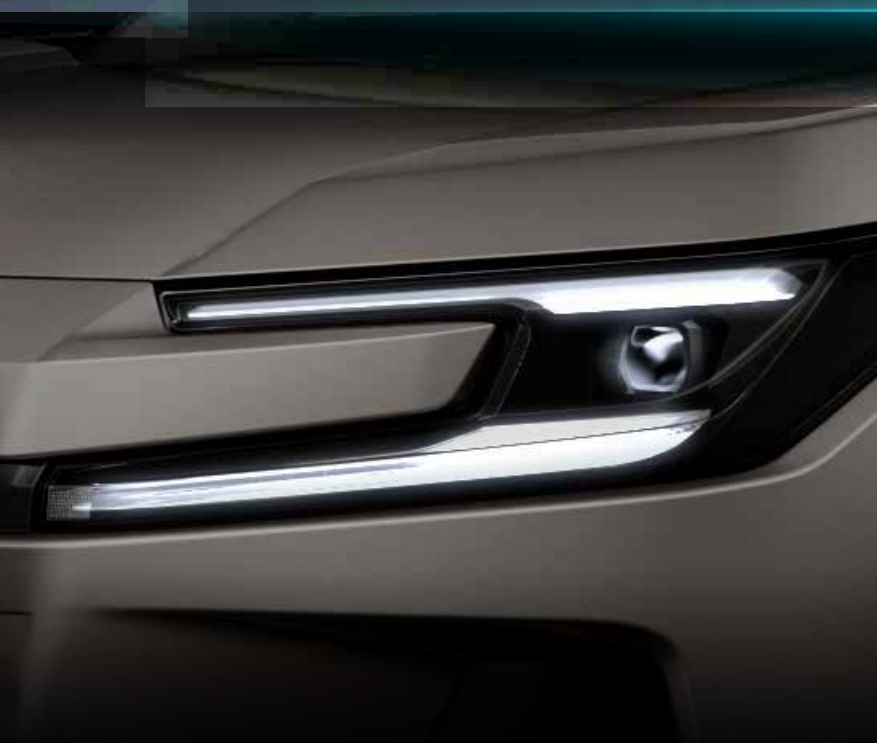
自動 Bi-LED 車頭燈附雙刃光條式日間行車燈 Auto Bi-LED Headlamp with Twin-Blade Day-Time Running Lamp
